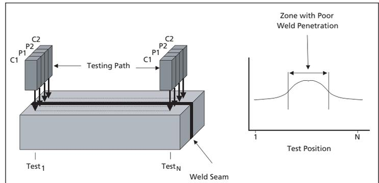
Figure 8: Series of Measurements Across a Weld Seam
