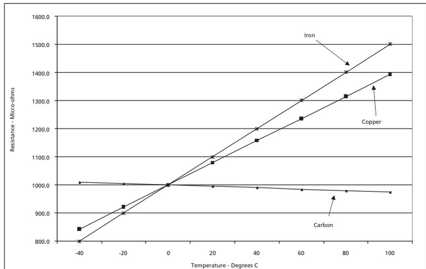
Figure 18: Temperature-Resistance Curves for Iron, Copper and Carbon
