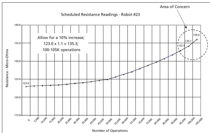
Figure 15: Trending Analysis of Low Resistance Readings
