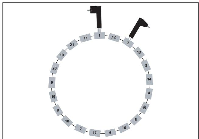
Figure 23 Coil Arrangement in a Wave Winding
