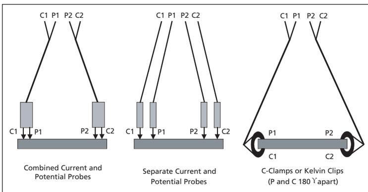
Figure 14: ProbelLead Configurations
