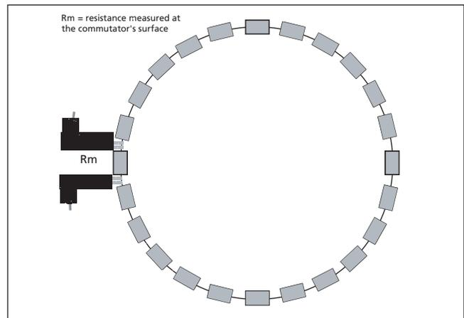
Figure 21: Commutator with 24 Coils in Series
