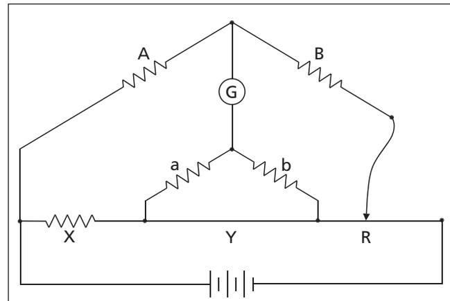
Figure 27: Kelvin Bridge Circuit<sup>viii</sup>
