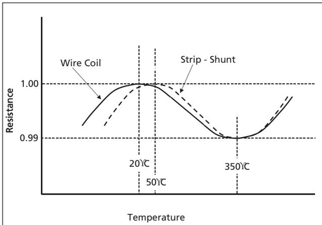
Figure 1: Qualitative Resistance-Temperature Curve for Manganin<sup>iii</sup>
