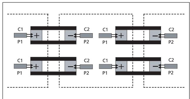
Figure 5: Parallel Straps on a Large Battery Complex
